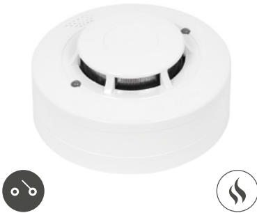
Optical Smoke Detector FDR26 Covered space: 40 m², max. height 7 m
