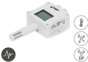
HTemp-485 T3411 Temperature range: -30 to 80°C, humidity range: 0–100% RH, dew point range: -60 to 80DP°C
