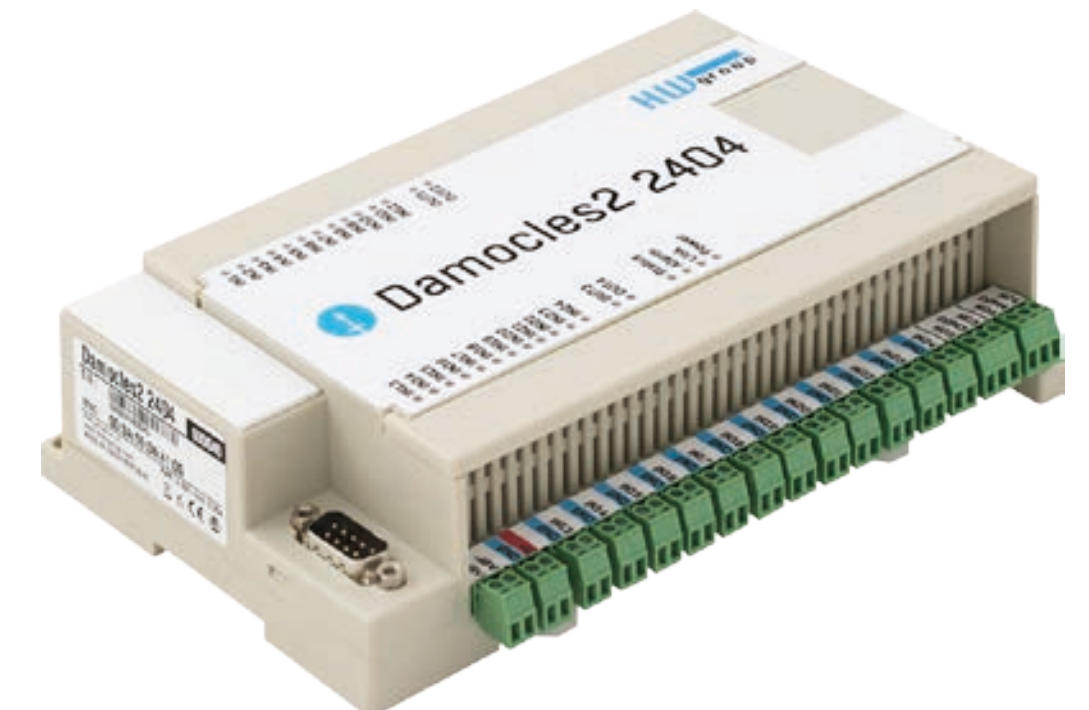
Damocles2 2404 Secure industrial I/O device with PoE and Telco -48 V power options.
